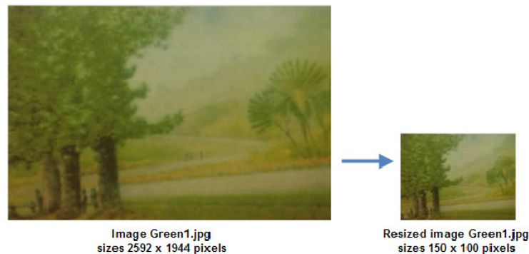
Figure 7. The illustration of resizing image
